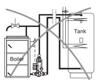
The pipe to the bottom of the tank must not be routed through the roof.
