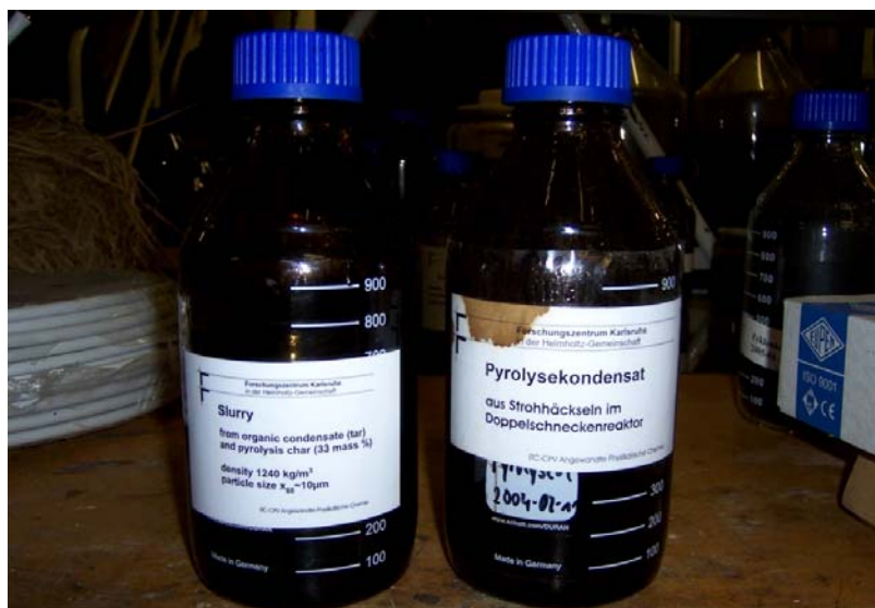
Figure 40: Slurry produced with the bioliq process
