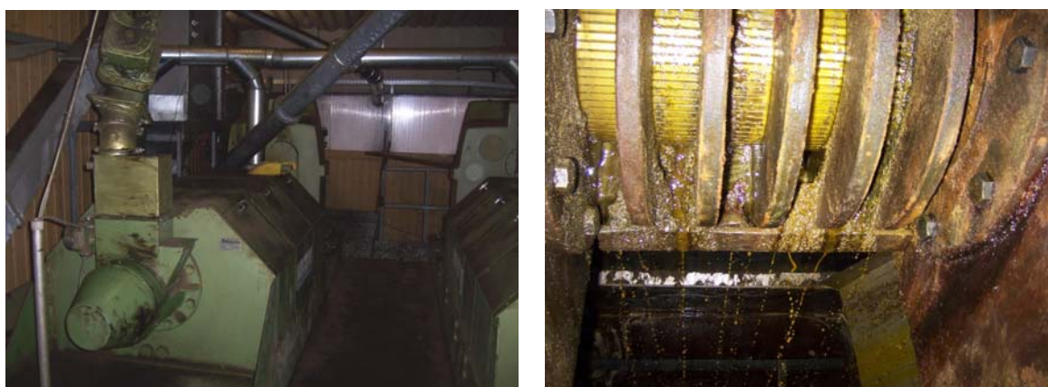
Figure 29: Small scale press for cold pressing of rape seed, Germany
