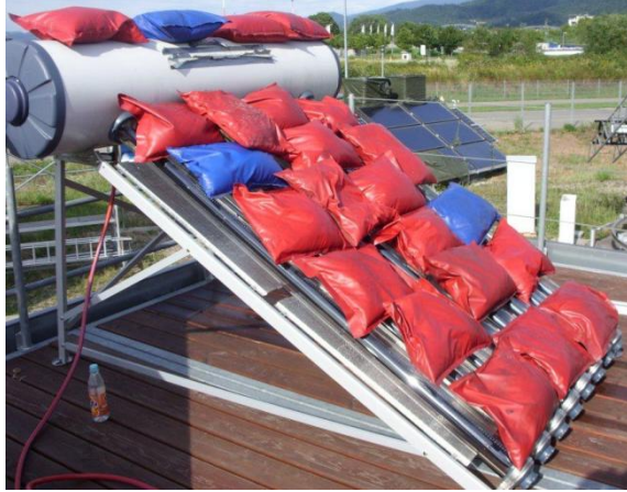
Figure 8: Example of a none separable system, mechanical load test with sand sack
