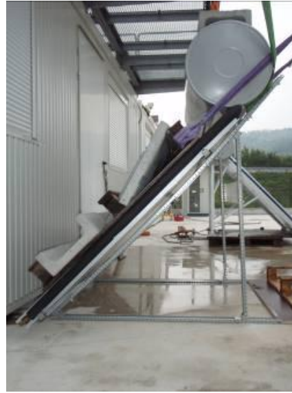
Figure 9 Example of a separable system mechanical load test with “stone load”.
